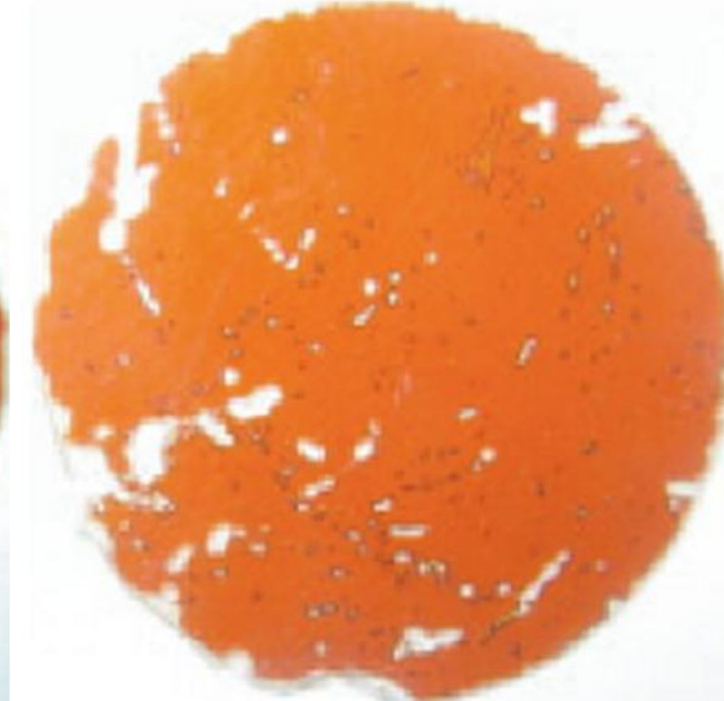
Figure 6: Kapton, shielded by DC93500 from AO/O3 (2)
